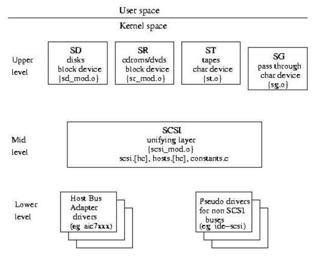
The 3 level driver architecture of the SCSI subsystem.
